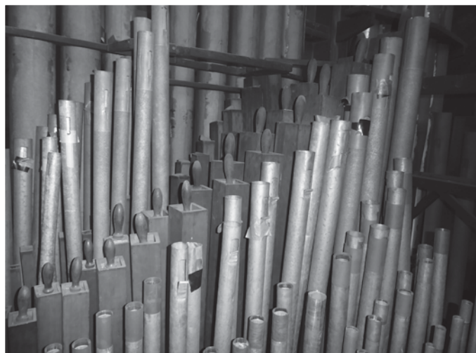
Pipes tuned by amateurs using duct tape and masking tape.
