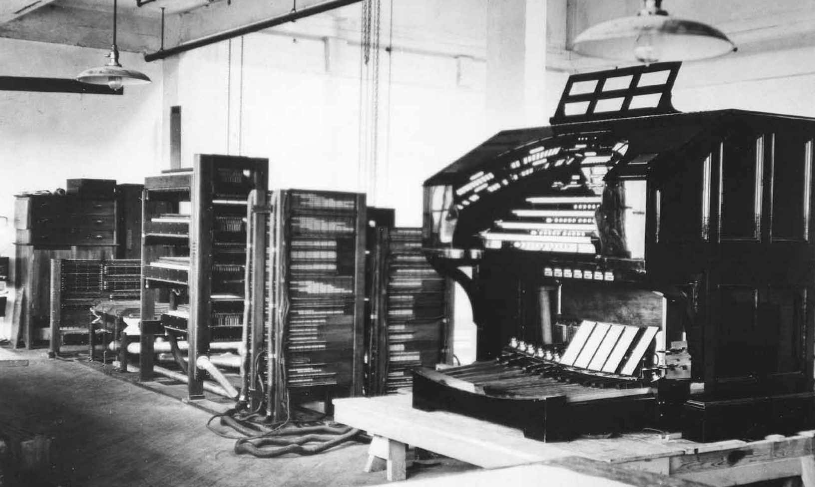
Above: The console and relay of the IV/32 Wurlitzer (Opus 138, 1917) for the Liberty Theatre in Portland, Oregon are set up for testing in the factory. This particular matrix-type relay, introduced by Hope-Jones, was among the last of this style to be built.
