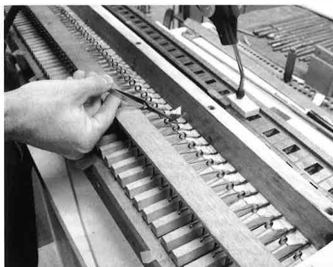
Using a syringe with a long tube extension, the conservator injects hide glue into the corners of the channels to stop leaks. He guides the syringe visually using a fiberscope. The directed treatment left serviceable original pallet leather unaltered. The conservator is Louis Dolive.
