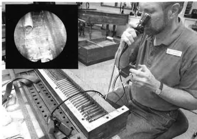
Using a syringe with a long tube extension, the conservator injects hide glue into the corners of the channels to stop leaks. He guides the syringe visually using a fiberscope. The directed treatment left serviceable original pallet leather unaltered. The conservator is Louis Dolive.
