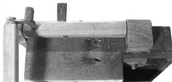
The shifting movement trundle with hand-forged iron arms, right pivot block, and sticker are all newly reconstructed. The work matches the style of the original, but each component is stamped with the date to make the reconstruction distinguishable. Modern saw marks left on the pivot block reinforce its origins. The trundle was made longer than the missing original, so the evidence of the original installation would remain untouched and visible.
