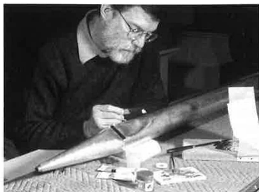
Localized gilding of the more distracting losses on the gilded facade pipes of the Wren Chapel organ minimized loss of historical evidence, and retained a legitimate appearance of age. The conservator is David Blanchfield.
