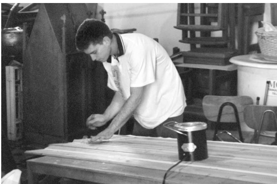
Markus Bansbach glues new leather hinges on wooden ribs of the wind reservoir.
