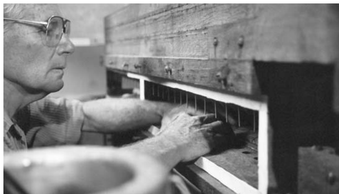
Peter Bansbach installs pull-down wires, dowels, and seals in a chest.
