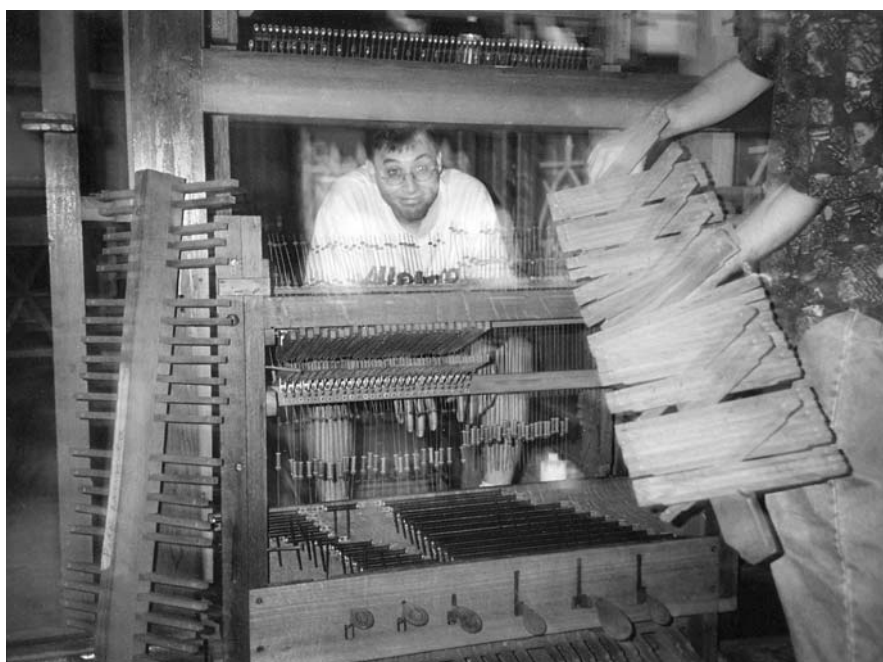
Jason Alden prepares to install a backfall as he and others re-erect the restored Schyven organ at Parroquia de Santo Domingo, Santo Domingo, Heredia.
