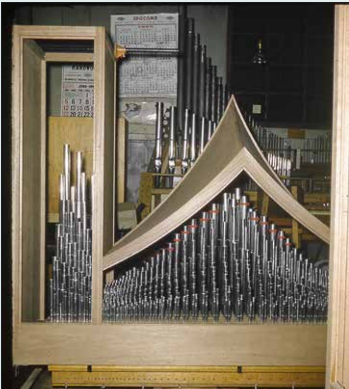
Workshop: Rugwerk case from behind, with pipes in place just after racking.
