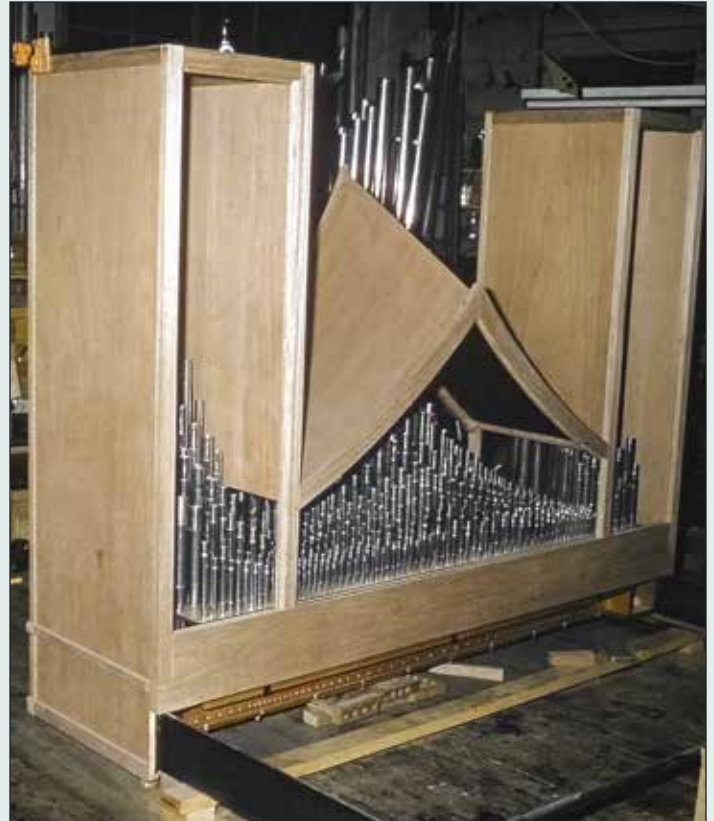
Workshop: Rugwerk case from behind, with pipes.
