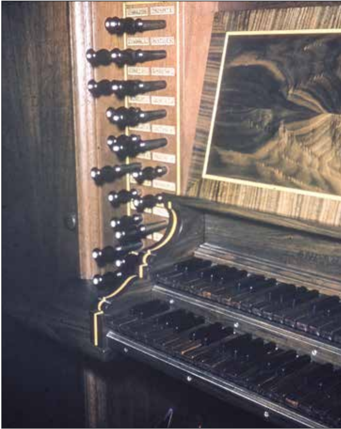
In Baltimore: Left stop jamb, with the original cocobolo naturals and ebony sharps. At bottom center, mechanical combination action pedals are just visible. Note oval ivory indicators on stopknobs, some of which are in vertical (OFF) position, others in horizontal (ON) position.
