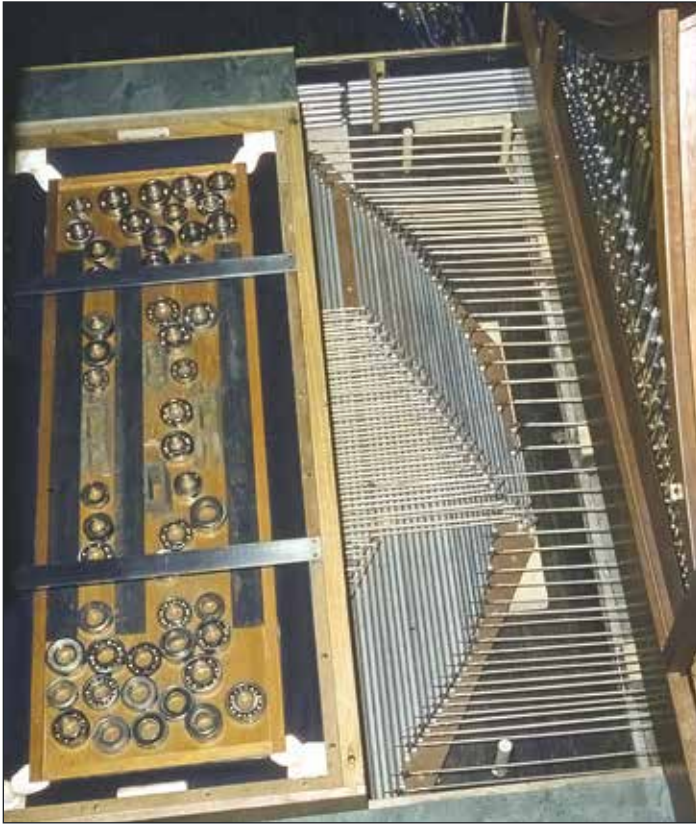
In Baltimore: Aerial view of Rugwerk wind regulator, rollerboard, and pipes. Mixture is in back row. Note the ball-bearing weights on the regulator.
