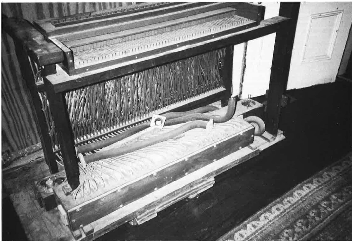
Remains of the Gustav Treu console from St. Stanislaus Church, St. Louis. The action was tubular-pneumatic to slider chests.
