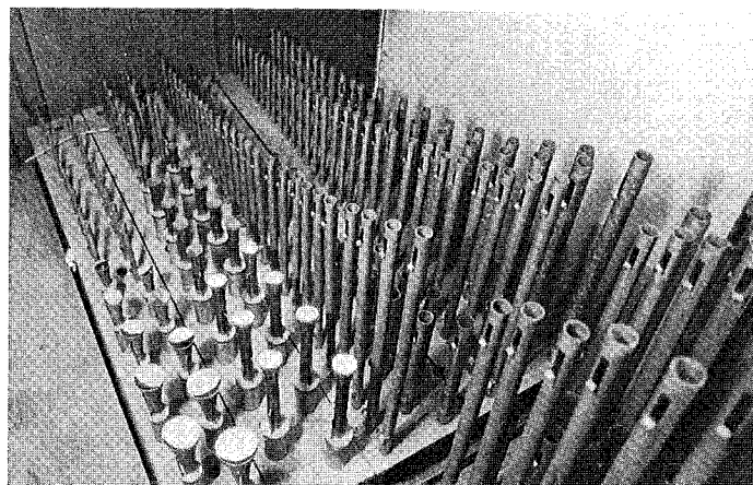
A photograph made before cleaning and restoration shows pipework on the upper Choir windchest, including the Violin Diapason at 4' pitch, where it was moved in 1960 but is now restored. Left to right: 4' Kopffregal, 8' Krummhorn of copper, 8' Aeoline, 8' Vox Coelestis, Violin Diapason, 8' Fernflöte.
