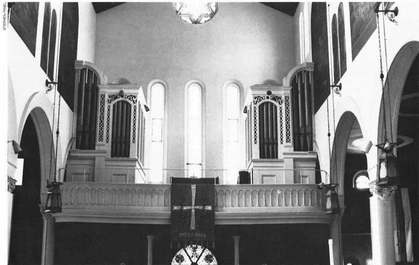
In 1941, St. Mary's R. C. Church, Newark, N.J., had Hillgreen, Lane & Co. saw its 1858 Ferris & Stuart (below) in half vertically and electrify its slider chests a second time, following Gustav Dohring's attempt in 1906.
