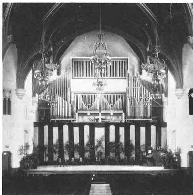
The 1925 E.M. Skinner organ at the University of Florida, Gainesville. Great and Pedal unenclosed; Swell, lower level; Choir and Solo, upper level.
