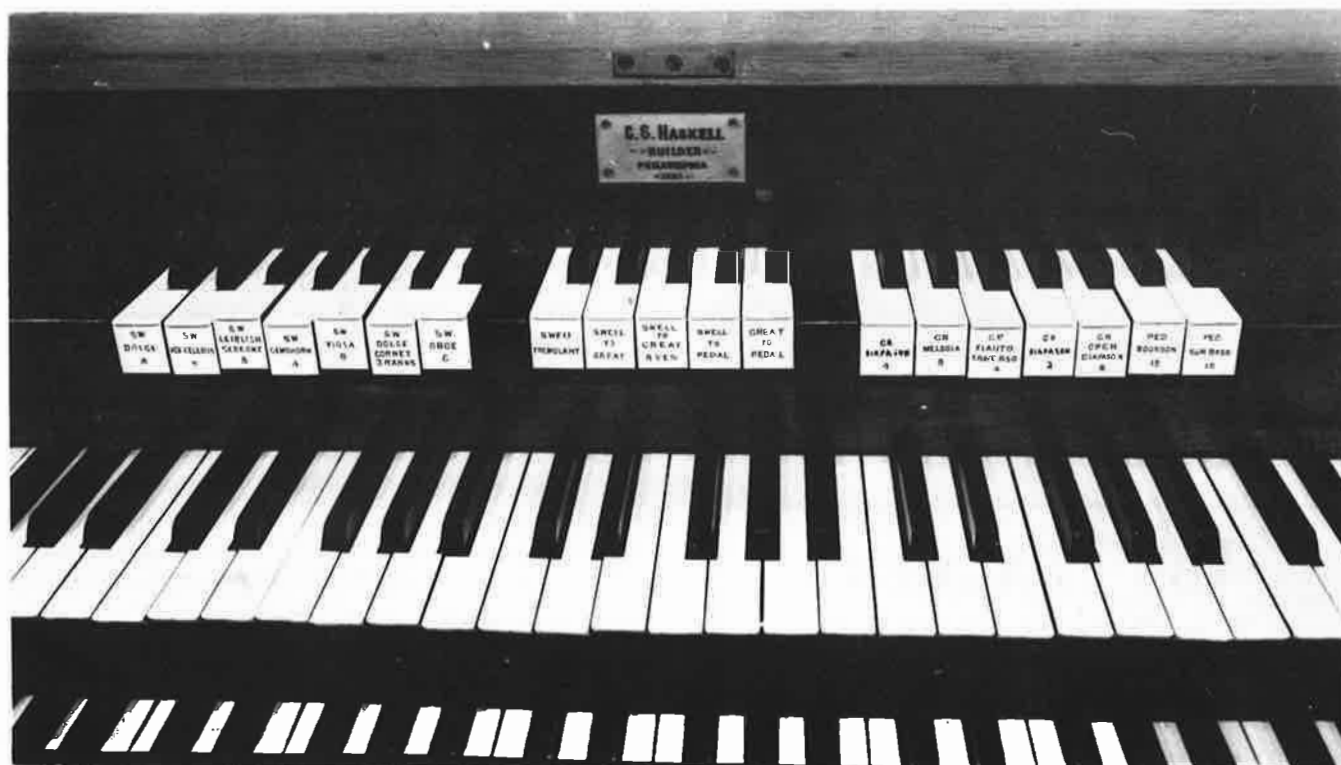
The Haskell organ features mechanical key action with pneumatic stop keys.
