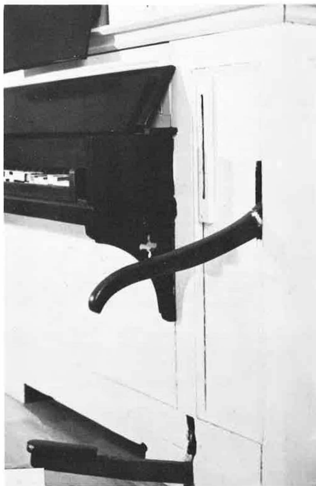
The pump handle and pedal, organ built by Wm. Metz, c.1846. Photo by Peter Pull.
