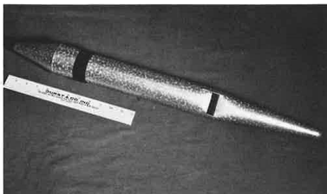
Number 12 (low B) pipe of 4' Koppelflote, showing characteristic shape. The length of the tapered part of the cap is important, as is the diameter of the smaller end of the cap, and whether that end is open or closed.
