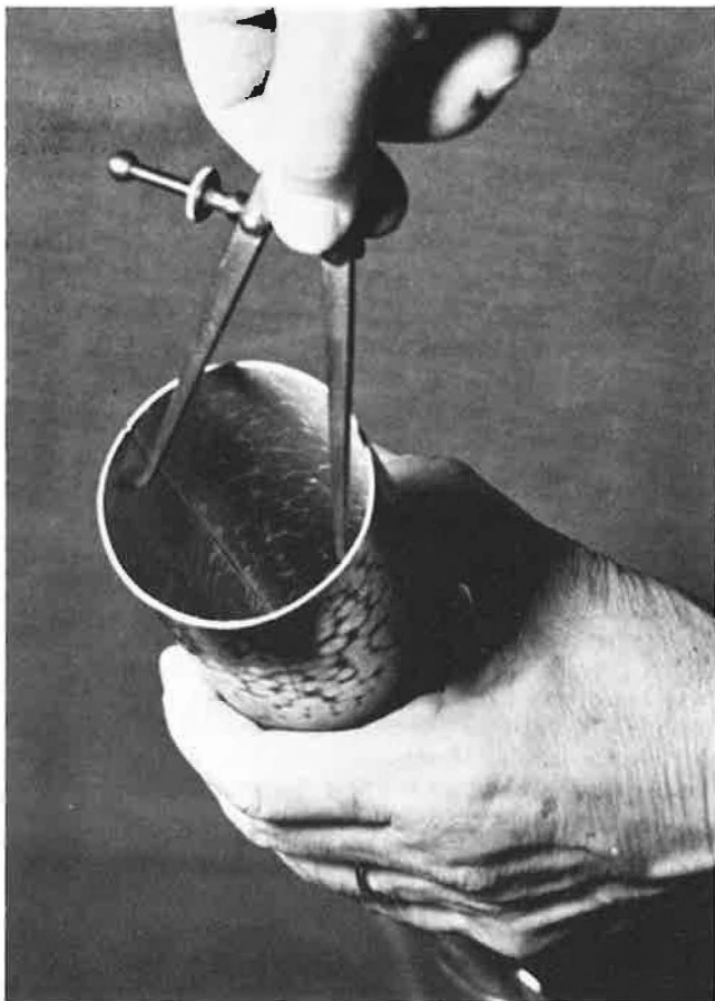
Measuring inside diameter of Koppelflote pipe with inside caliper.
