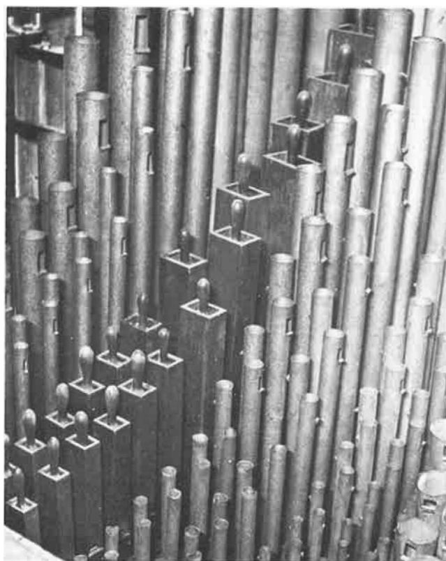
The great organ pipework showing the famous Doppelflote. Note cone tuning on flues in foreground.
